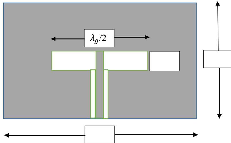
Fig. 1. Geometry of the proposed antenna fed by CPW. (Dimensions are in mm.)
