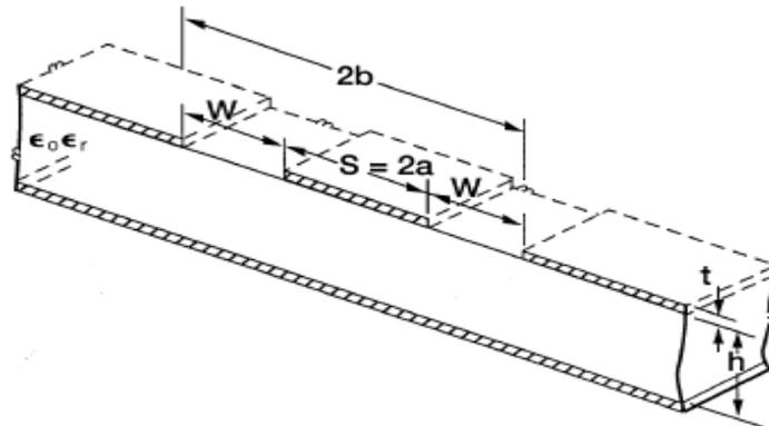
Fig. 2. Schematic of conductor Backed Co-planar Waveguide
