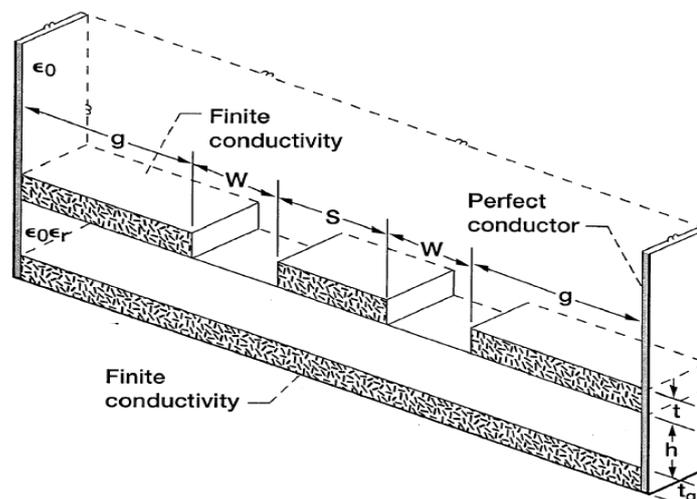
Fig. 3. Schematic of conductor Backed Co-planar Waveguide with finite thickness
