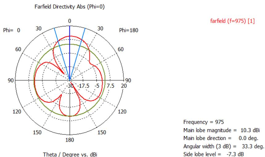
Fig.5 Directivity of antenna
