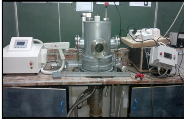
**Figure 1.** Pulsed laser deposition (PLD) system.
