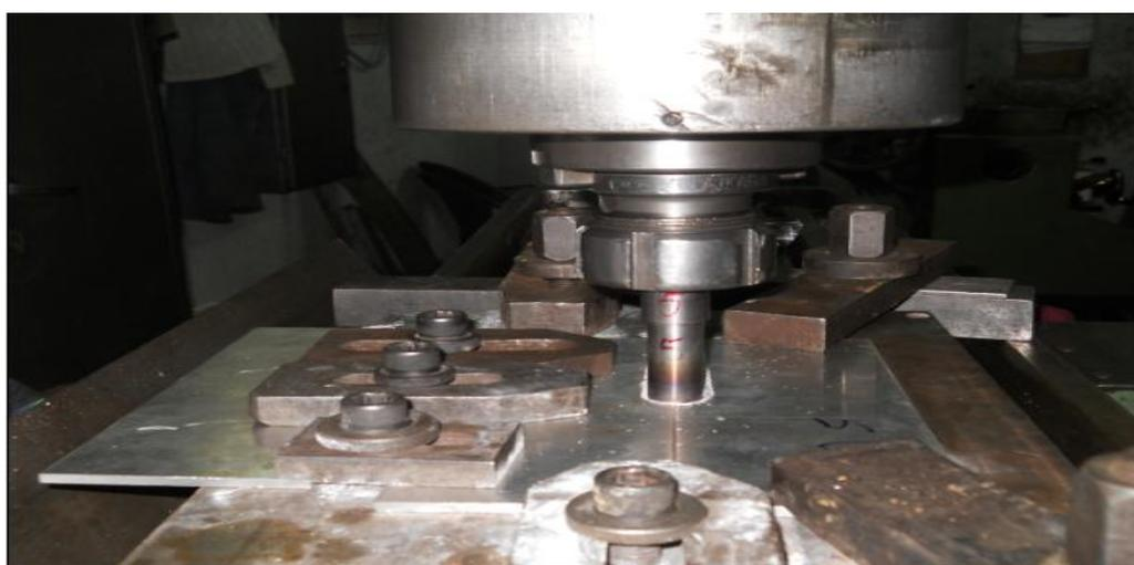
**Figure 1: Friction stir welding experimental set-up**
