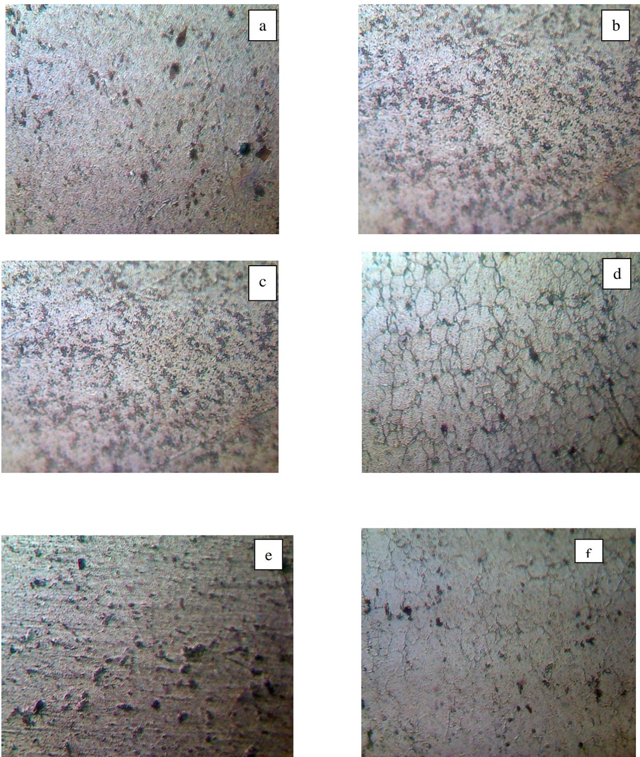
**Figure 3: Optical microstructures of (a) base material (b) FSW samples of straight cylindrical tool, (b) taper cylindrical tool (d) threaded cylindrical tool (e) square and triangular tool (f) square and triangular tool**
