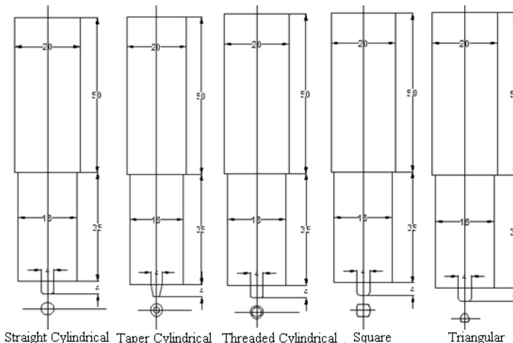
Figure 2: FSW tool pin Profiles
