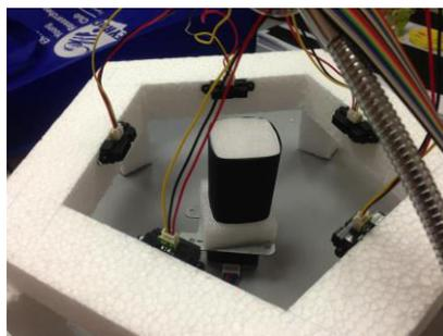
Fig. 2 The arrangement of sensor rig with an object located at the centre of the IR.
