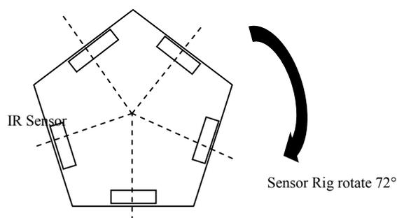
Fig. 1 Arrangement of sensor rig and IR sensor position
