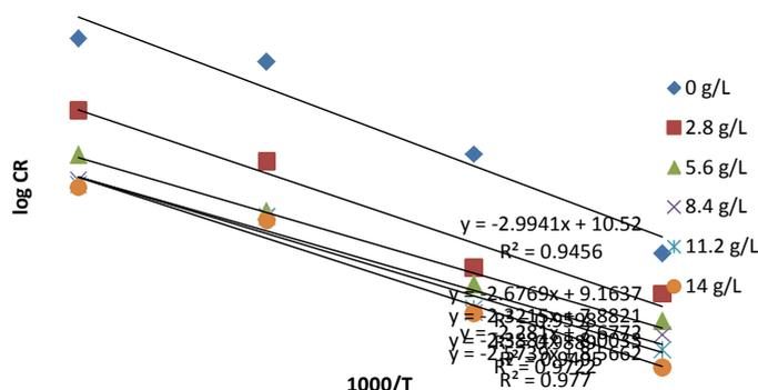
**Figure 4.** Arrhenius plot for Al dissolution in 1.0M NaOH with and without of (CD) extracts after 1 h immersion time.
