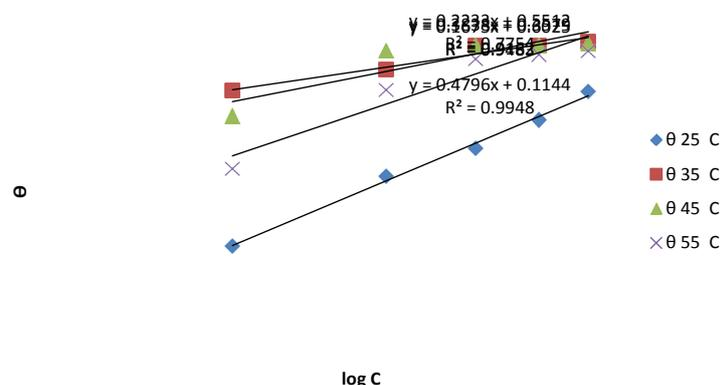
Figure 6. Temkin adsorption isotherm plot ( $\theta$  against  $\log C$ ) for Al in 1M NaOH with (CD) extract after 1 h immersion time at different temperatures.
