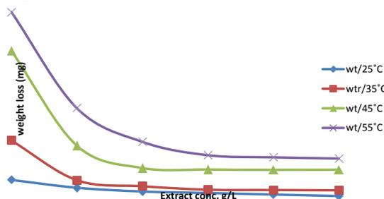
**Figure 2.** Variation of the weight loss of Al metal versus (CD) extract concentration in 1M NaOH at different temperatures after 1 h immersion time.
