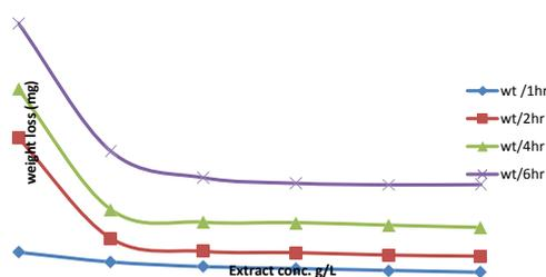
**Figure 1.** Weight loss variation of Al metal versus (CD) extract concentrations at 25°C in 1 M NaOH at different immersion times.
