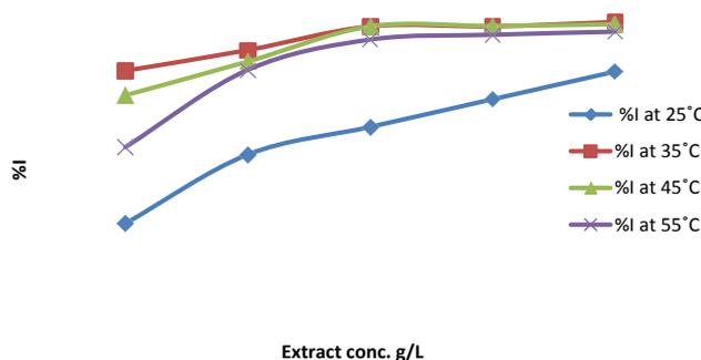
**Figure 3.** Inhibition efficiency versus (CD) extracts concentrations for aluminum in 1M NaOH at different temperatures after 1 h immersion time.
