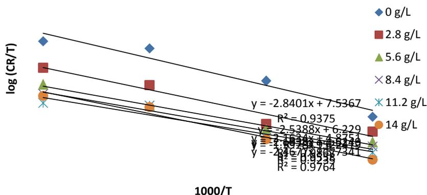
**Figure 5.** Log (CR/T) vs.  $1000 \times 1/T$  for Al in 1.0M NaOH in the with and without of (CD) extract after 1 h immersion time.
