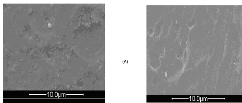
Figure 7. Scanning electron micrographs of (A) aluminum surface in 1.0M NaOH solution, (B) aluminum surface in 11.2 g/l of (CD) extract concentration.
