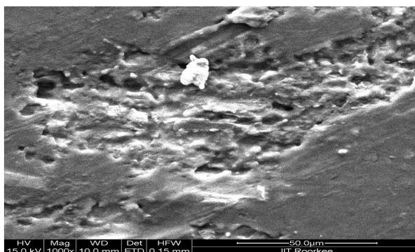
Figure 11: SEM of copper immersed in 0.5 N HCl inhibitor containing 1.052 g/L resulting highest IE % (97.72).
