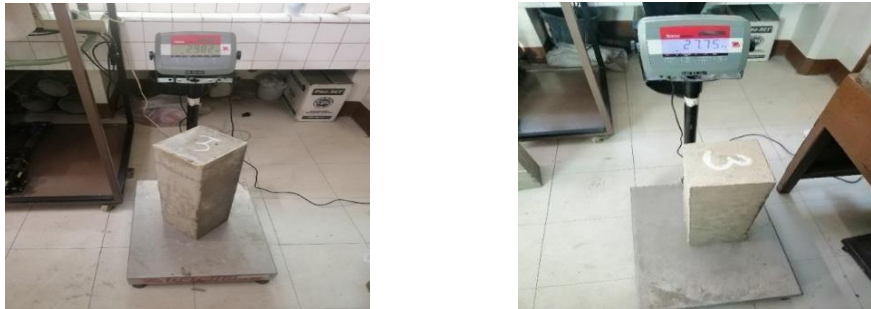
Figure 4: Weight of Conventional Concrete sample and Glascrete sample
