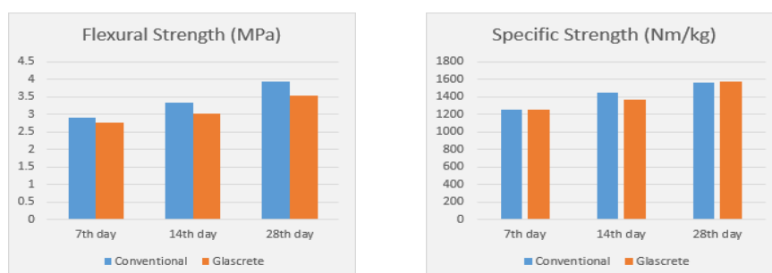
Figure 3: Flexural strength and specific strength of the rectangular samples.
