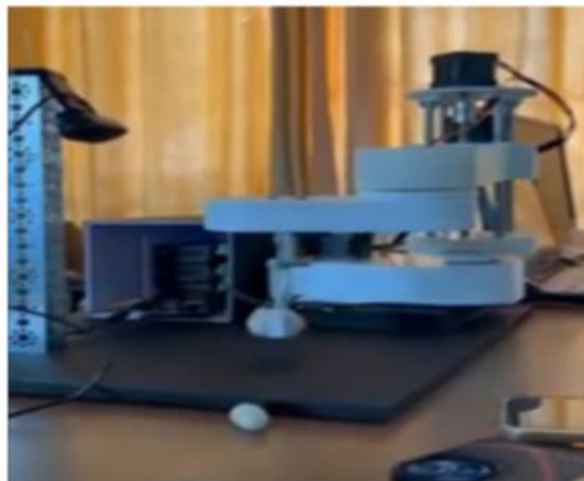
Figure 5. 3-DOF SCARA Robot.
