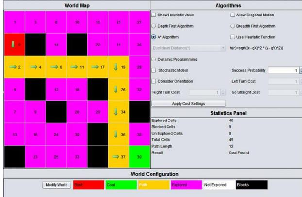
Fig. 4 Exploration of A\* algorithm without heuristic values
