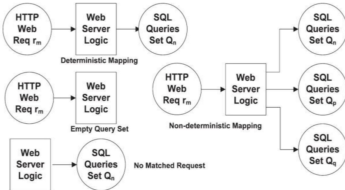
**Figure.6 Representation of Mapping Patterns**
