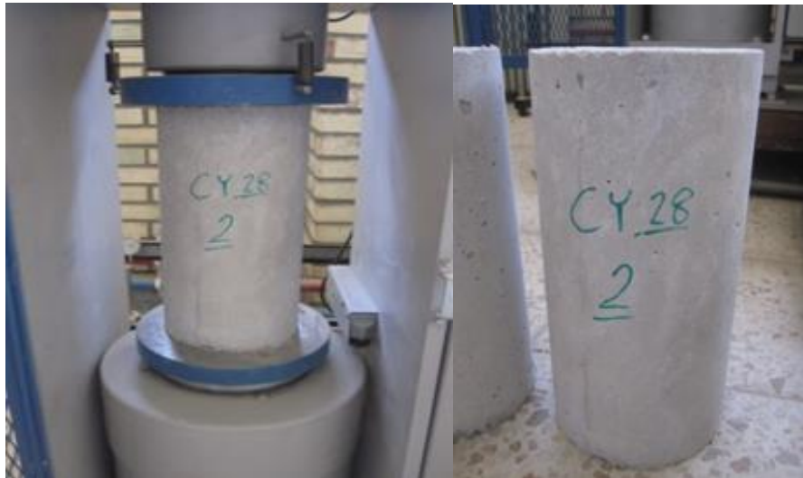
Figure 3: Sample CY A2 before compressive strength testing
