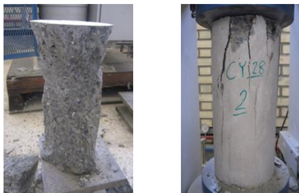
Figure 2: Sample CI A2 under the 28-day compressive strength
