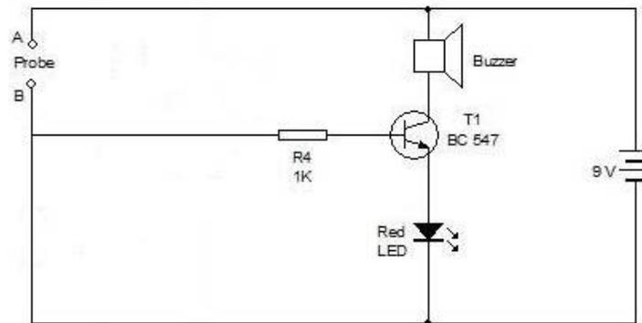
Fig. 1. Circuit of existing Tank Overflow Control Model
