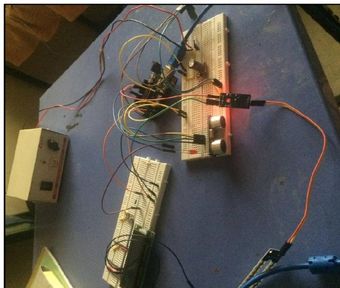
Fig. 6. Circuit for Smart Irrigation and Tank Monitoring System
