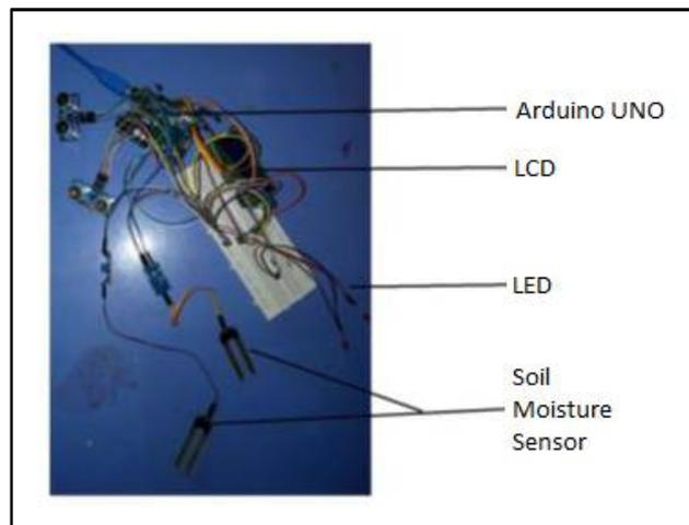
Fig. 3. Circuit for Soil Moisture Monitoring Module
