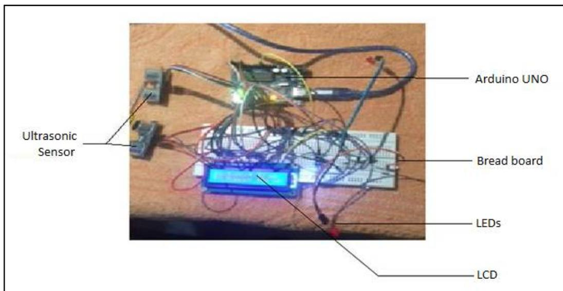
Fig. 4. Circuit for Tank Monitoring Module
