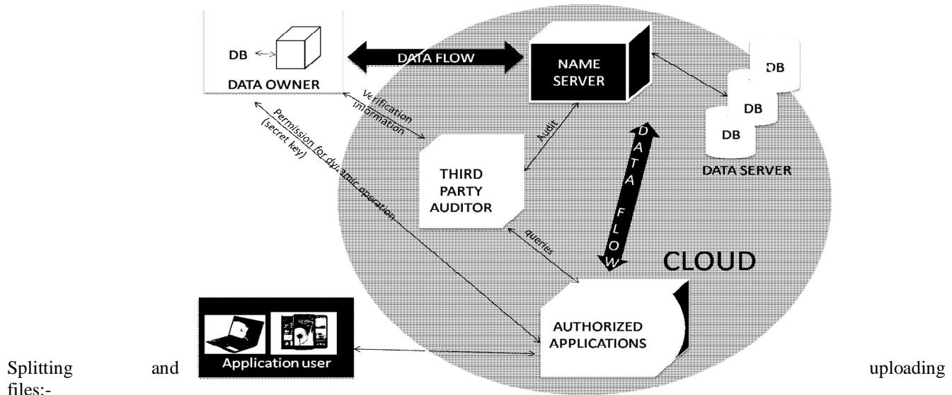
File splitting is an approach to protecting sensitive data from unauthorized access by encrypting the data and storing different portions of a file on different servers.
