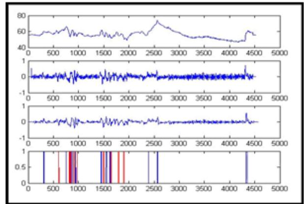
Figure 2 Signal trace from the Artificial Neural Network study showing a response to a number of stressful situations (top), normalized difference (mid top), filtered difference (mid bottom) and negative (red) and positive (blue) thresholds (bottom). The thresholds can be set at different trigger levels to provide a gauge to the number of various-intensity stress or emotion response peaks that occur over a period of time.
