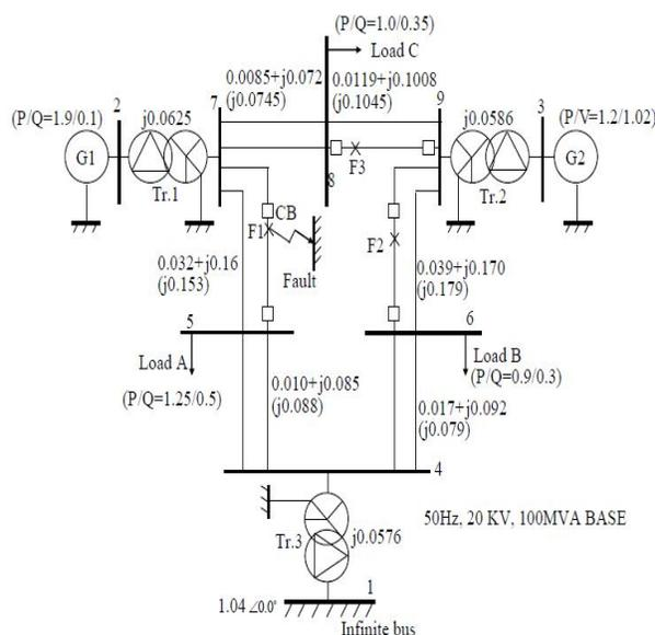
Fig.1. IEEE nine bus power system model.
