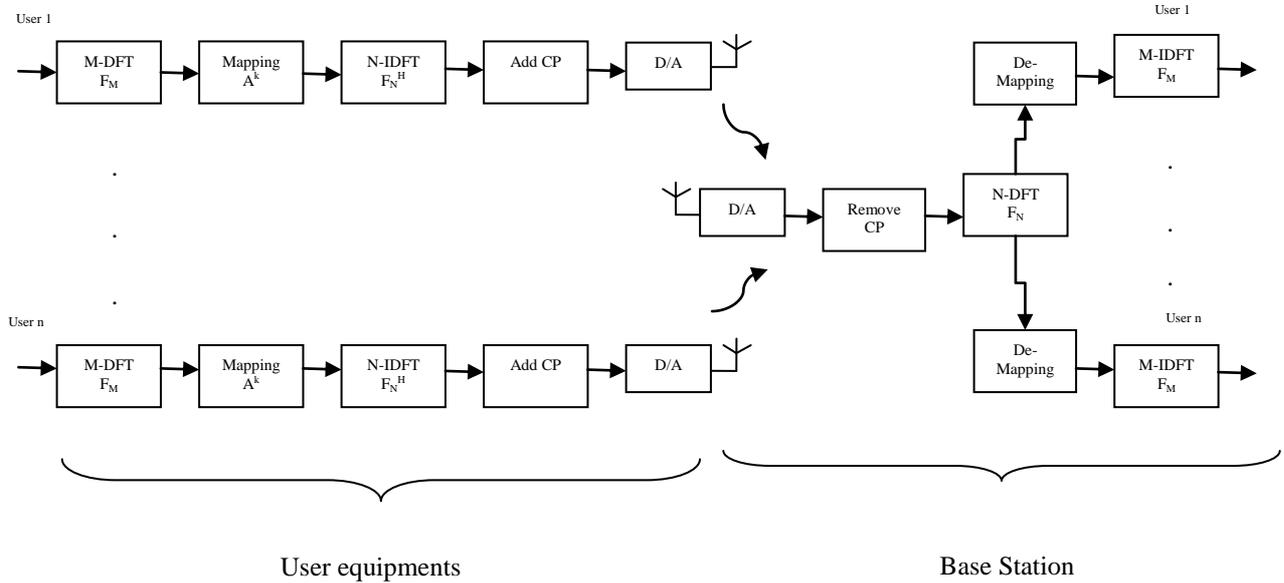
Fig.1 Uplink SC-FDMA System Model
