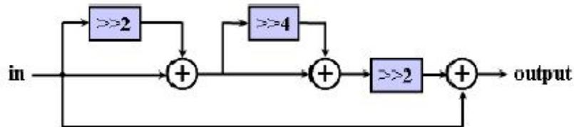
Fig.1: Circuit diagram of the bit-parallel multiplication by 1/ sqrt (2)
