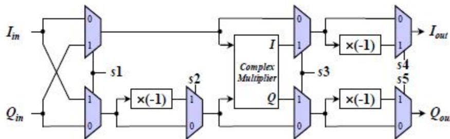
Fig.3: Reconfigurable complex constant multiplier
