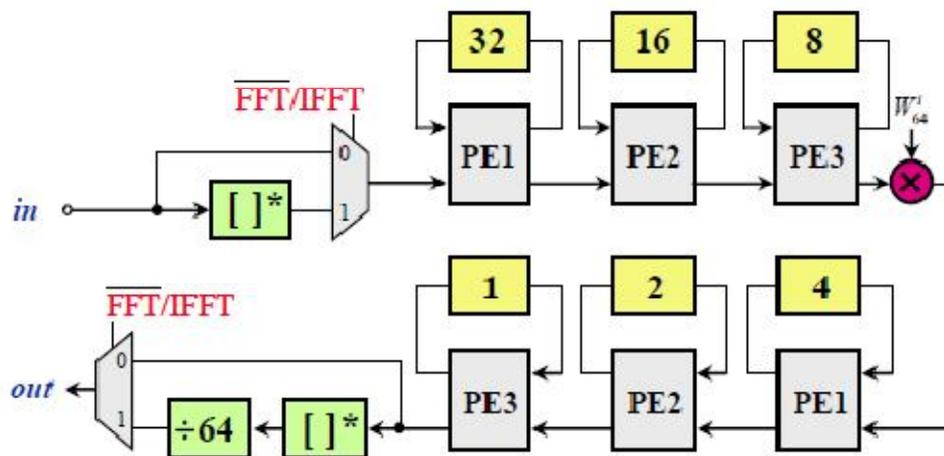
Fig.7: Proposed radix-2 64-point pipeline FFT/IFFT processor.
