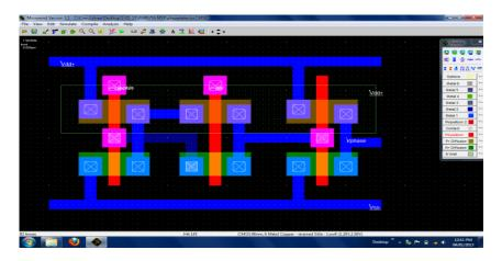
Figure 7.Layout of Loop filter
