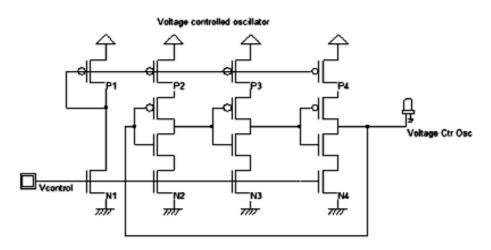
Figure 9.CMOS circuit of VCO
