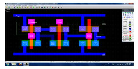
Figure 4.Layout of Phase Detector
