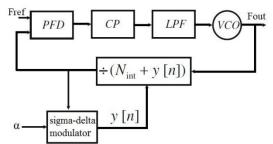
Figure 2. Block Diagram of PLL using Sigma-delta fractional -N frequency synthesizer
