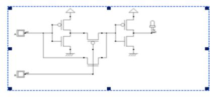
Figure 3.CMOS circuit of Phase Detector
