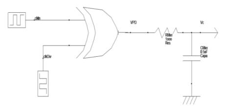
Figure 6.CMOS circuit of Filter
