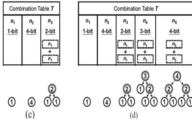
(c) New combination  $n_3$  is obtained from combining two  $n_1$ s. (d) New combination  $n_4$  is obtained from combining  $n_1$  and  $n_3$ , and the combination  $n_5$  is obtained from combining two  $n_3$ s.
