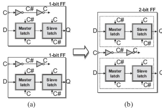
Fig. 1. Example of merging two 1-bit flip-flops into one 2-bit flip-flop.
