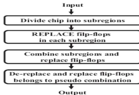
Fig 5 detailed flow to merge flipflops
