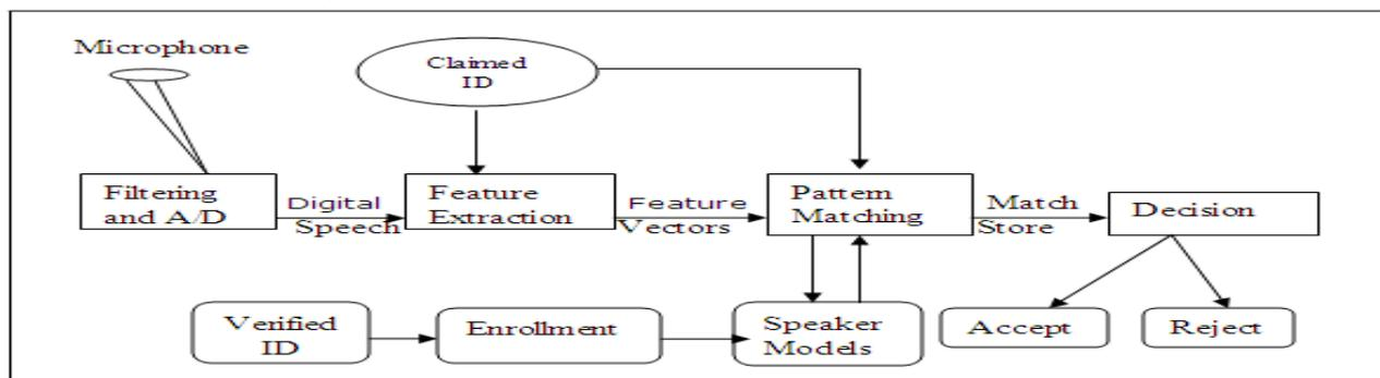
Fig: 1:- Speech recognition automation architecture
