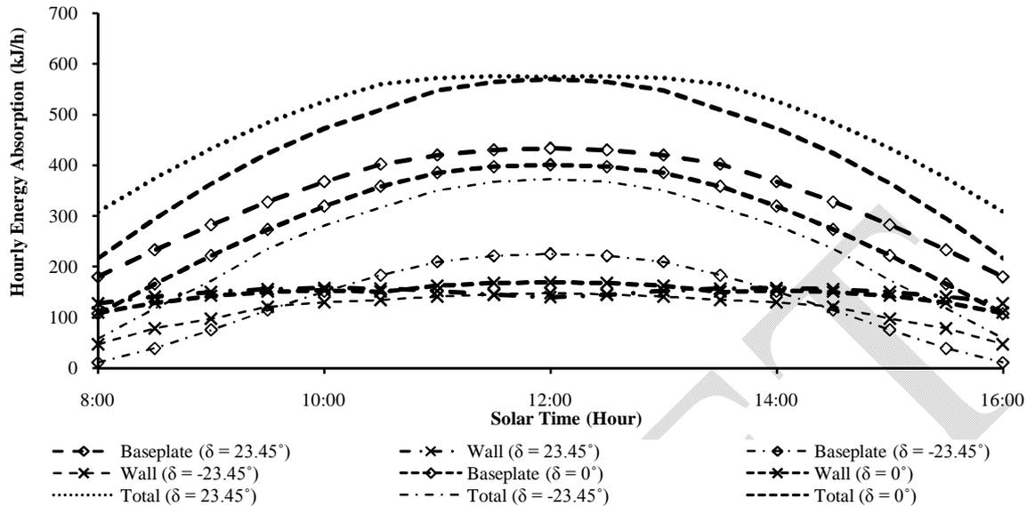
Fig. 4. Variation in hourly energy absorbed by the base plate and walls of the solar collector for global radiation for three declinations ( $\delta$ )
