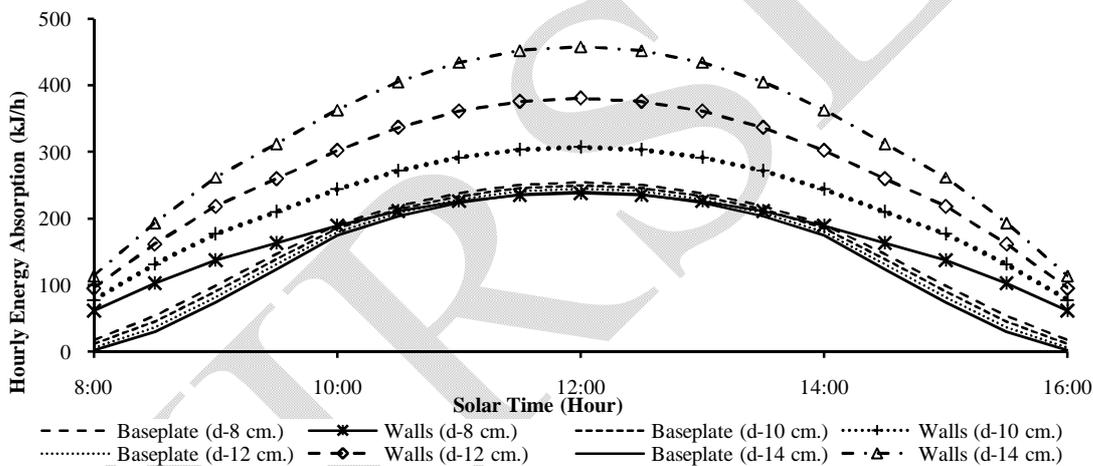
Fig. 7. Variation in hourly energy absorbed by the base plate and walls of the solar collector for different wall heights (d) but fixed wall inclination ( $\theta_w = 40^\circ$ ) for global radiation on Dec-21
