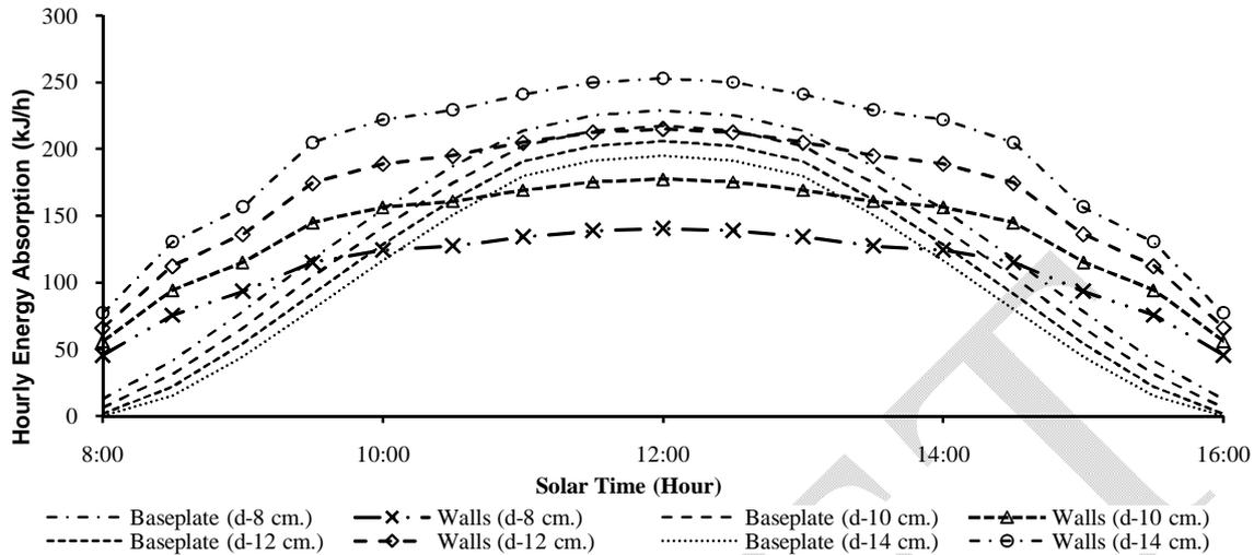
Fig. 6. Variation in hourly energy absorbed by the base plate and walls of the solar collector for different wall heights (d) but fixed wall inclination ( $\theta_w = 20^\circ$ ) for global radiation on Dec-21
