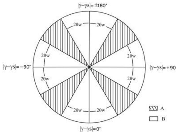
Fig. 3. Conditions of  $|\gamma - \gamma_s|$  showing shading of one wall (B)/two walls (A) completely. Area 'A' in the figure represents the shading of two adjacent walls completely and partial shading of the other two walls, and the area 'B' represents the shading of one wall completely and partial shading of walls adjacent to the shaded wall.
