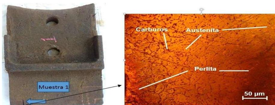
The microstructure is based on an austenitic matrix, which has precipitated carbide compounds and small pearlite colonies, which is the result of the rejection of carbon by the austenite during cooling. These carbides have nucleated at the grain boundaries and in the interdendritic areas within the austenite grains. They do not have a massive character and presumably are of the  $M_xC$  type, exposed [10].
