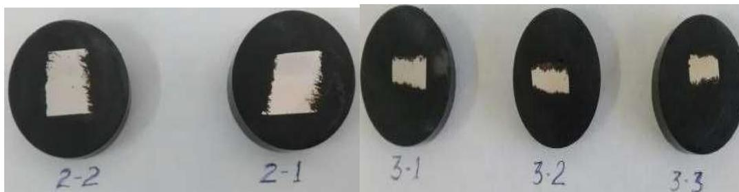
**Roughing and polishing:** Once the samples were placed in the phenolic container, they were roughed, which, roughly speaking, consisted of first obtaining a flat and semi-polished surface, using machine tools and abrasive papers. Polishing was carried out, guaranteeing a variation of the grain size from the coarsest to the finest.
