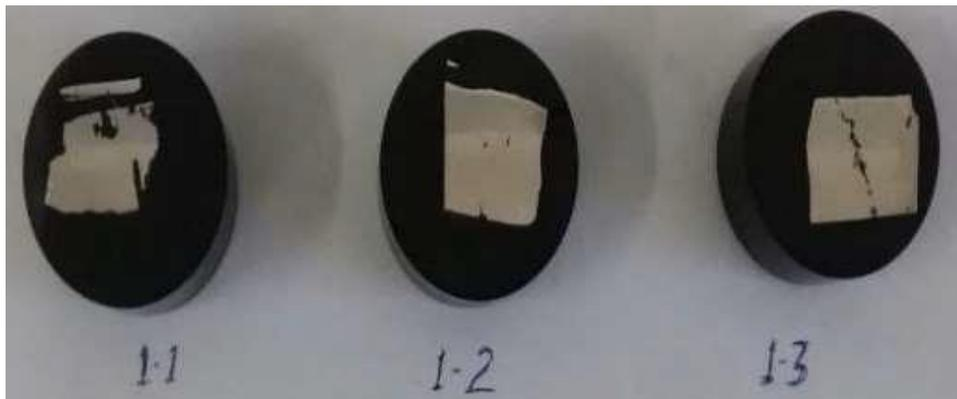
**Figure 4.** Encapsulated samples of the alloys out of service.
