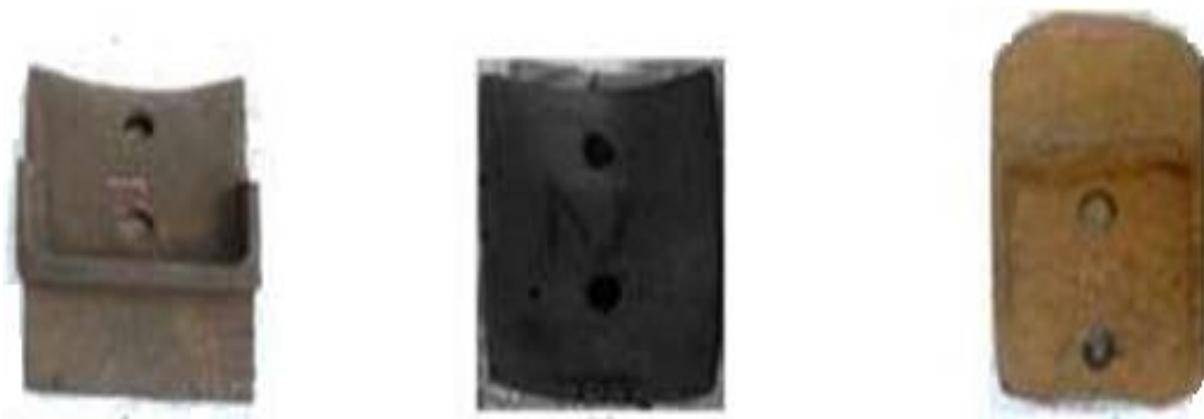
The specimens were cut (Figures 2a and 2b), with the use of a cutting disc, with abundant cooling to avoid heating due to friction effect, because the temperature produced can alter the structure, at least on the surface obtained [7].
