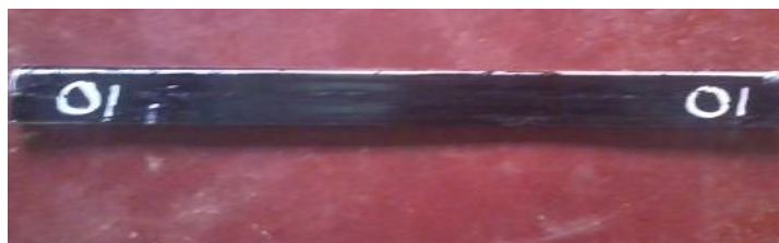
Fig. 1 Composite with 0% fiber prepared using Hand layup procedure
