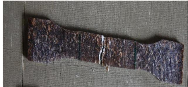
Fig. 1 A sample Specimen after Tensile Test
