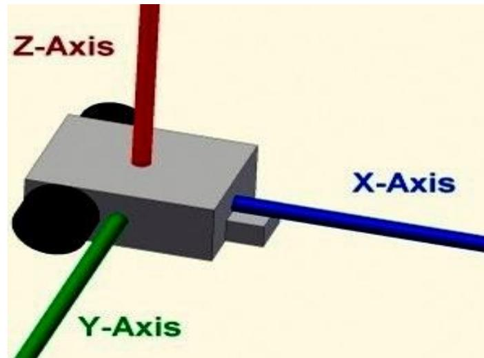
Fig. 1 Sensing direction of the triaxial MEMS accelerometer
