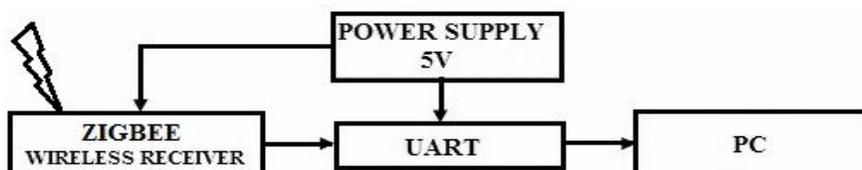
Fig. 3 Block diagram of receiving module
