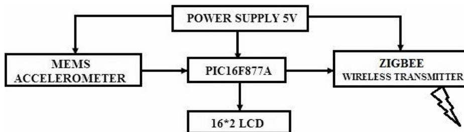
Fig. 2 Block diagram of transmitting module
