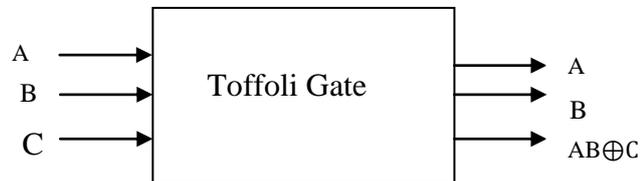
Figure.5 Block diagram of Toffoli Gate
