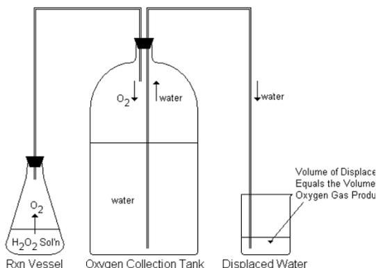
Fig. 1 Experimental setup to determine the rate of decomposition with the addition of catalyst [1]
