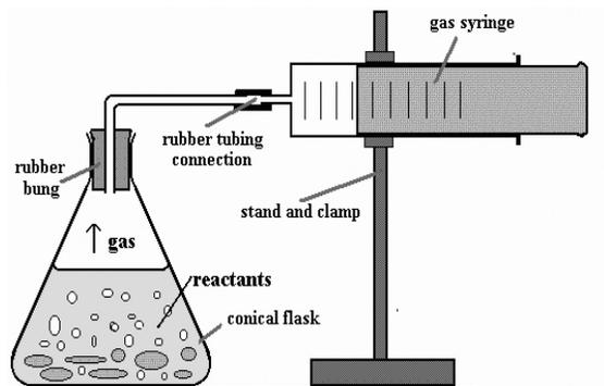
Fig. 2 Experimental setup to determine the rate of decomposition without the addition of catalyst
