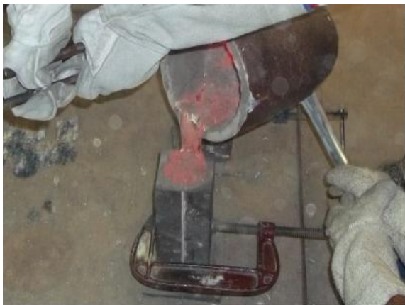
Plate.2.7 Pouring and solidification to produce die castings
