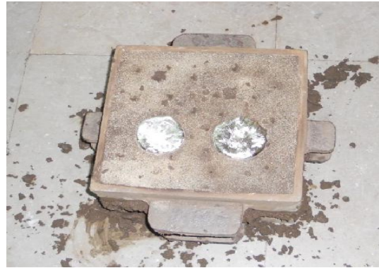
Plate.2.6 Pouring and solidification to produce sand castings.
