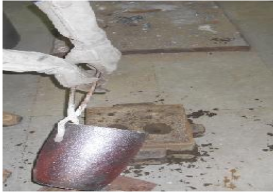
Plate.2.6 Pouring and solidification to produce sand castings.
