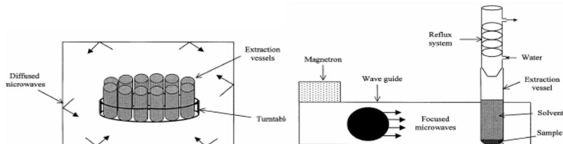
Figure 1. Scheme of the two microwave systems, using diffused or focused microwaves.
