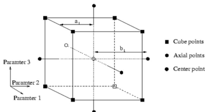
Figure 4. Distribution of experimental points in a three variable central composite design.
