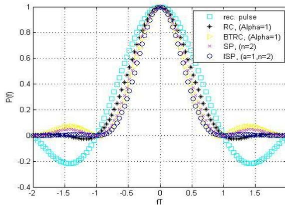
Fig 4: Spectral representation of various Pulses
