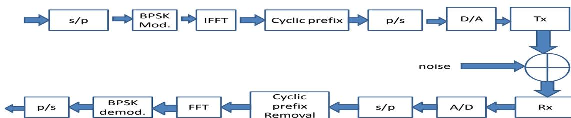
**Fig 1: A simple block diagram of MIMO OFDM System**
