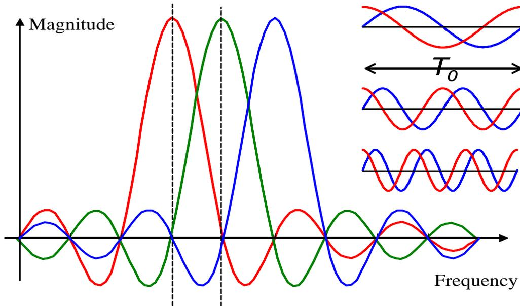
Fig 2: Magnitude versus Frequency curve of an OFDM symbol
