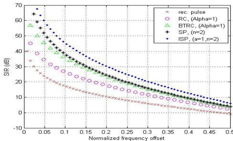
**Fig 7 SIR Performance for Different Pulse Shapes**
