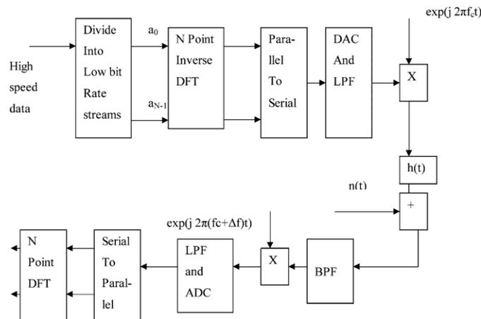
Fig 3: An OFDM system proposed with Pulse Shaping
