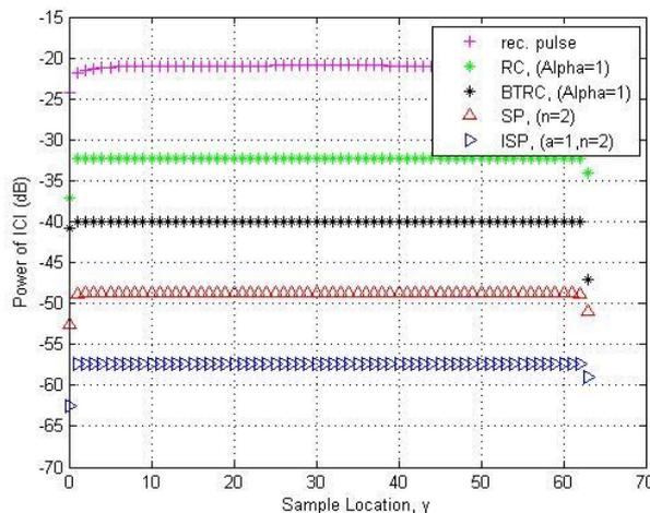
Fig 5: Comparison of ICI power of different Pulses
