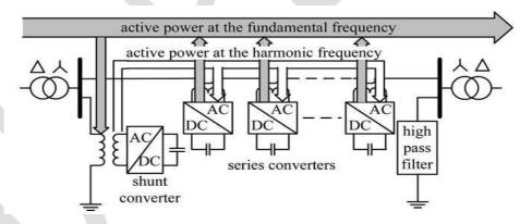
Fig. 2. Active power exchange between DPFC converters.
