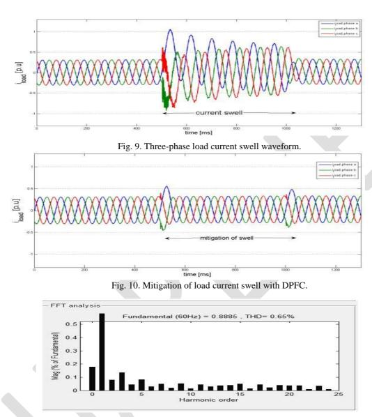
Fig. 11. The load voltage THD.
