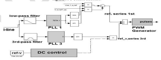
Fig. 4. The series control structure.
