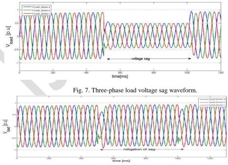
Fig. 8. Mitigation of three-phase load voltage sag with DPFC.
