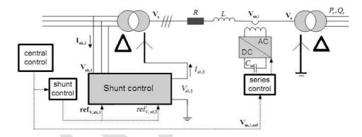
Fig .3.DPFC Control Structure.
