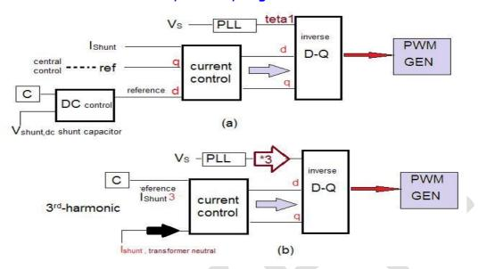
Fig. 5. The shunt control configuration: (a) for fundamental frequency (b) for third-harmonic frequency
