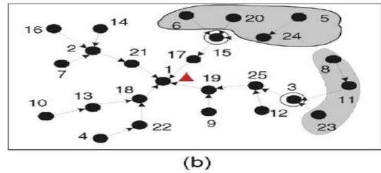
sensor 1 denoted by  $T'$ , is depicted in Fig.3a. In the first iteration, sensor 8 is found to be farthest leaf vertex on  $T'$  with five hops away from the root, that is,  $v=8$ . Its two hop parent vertex  $u$  on current  $T'$  is sensor 3 ( $u=3$ ), which will be marked as PP.
