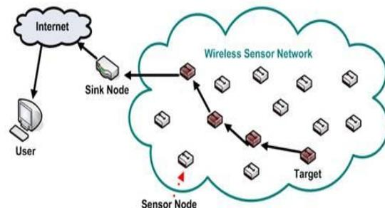
Acquired information is wirelessly communicated to a base station (BS), which propagates the information to remote devices for storage, analysis, and processing.
