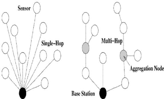
Figure 2 Single-Hop and Multi-Hop transmission
