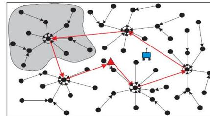
● Sensor → Relay routing path → Mobile collector tour
