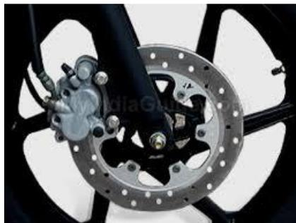
**Fig.1** Assembly of Disc Brake
