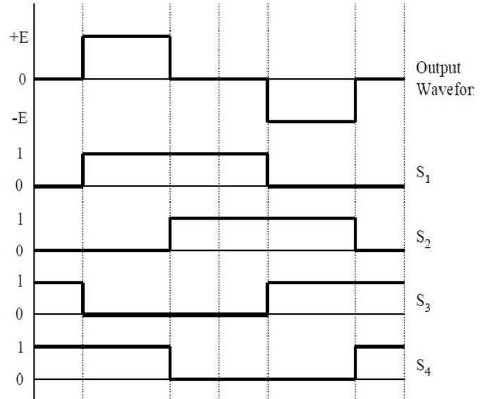
Fig 2. Repeated zero level switching pattern
