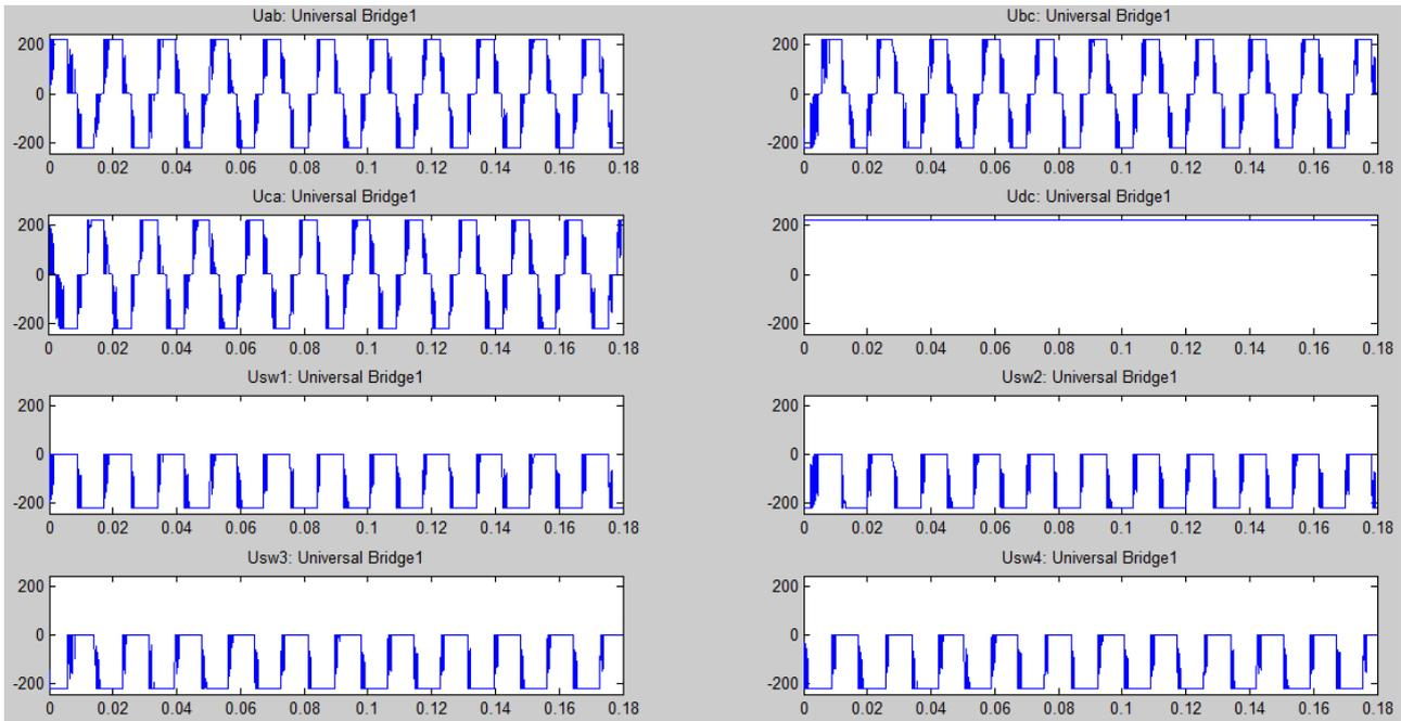
Figure 3: Converter bridge wave form for supply voltage, dc bus voltage.
