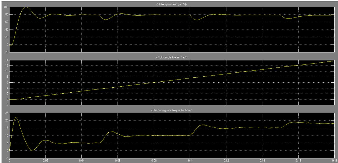
**Figure 8:** Rotor speed, Rotor angle and Electromagnetic –Torque wave form.
