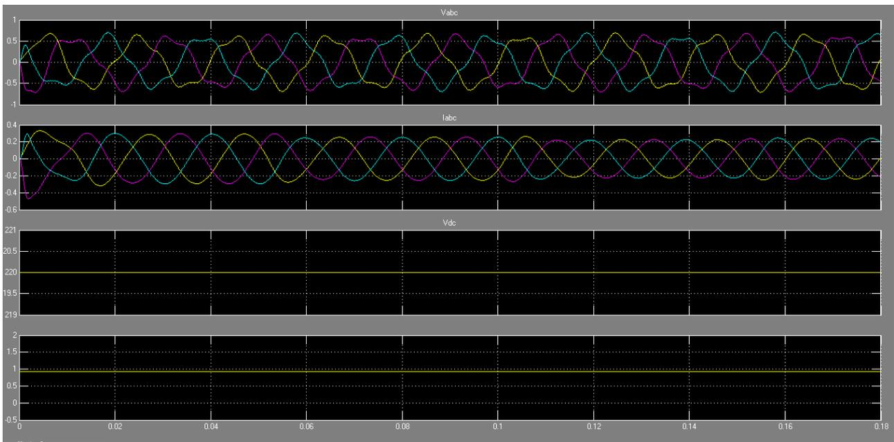
Figure 4:  $V_{abc}$ ,  $I_{abc}$ ,  $V_{dc}$  to Inverter and MI value of Converter bridge wave form.
