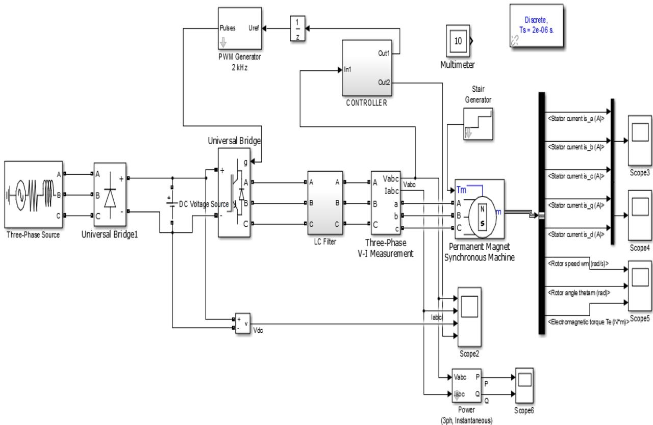
Figure 2: Simulation of main circuit.
