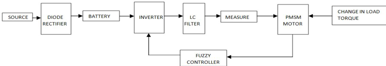
Figure 1: Circuit diagram of proposed PMSM motor drive.
