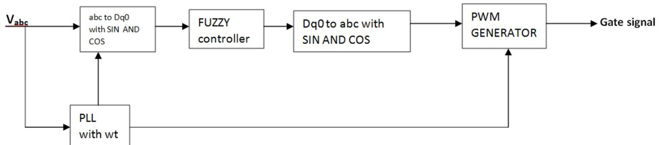
Figure 1a: Circuit diagram of Controller used in PMSM motor drive.
