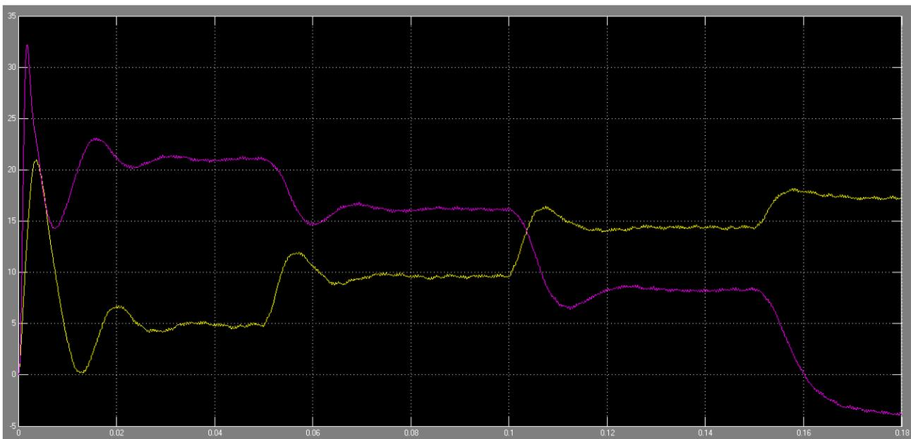
Figure 7: Stator  $I_q(A)$  and  $I_d(A)$  currents waveform.
