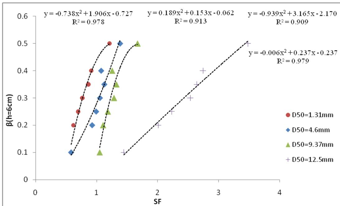
Figure 6: longitudinal shear force at different roughness in ( $h = 6\text{cm}$ )
