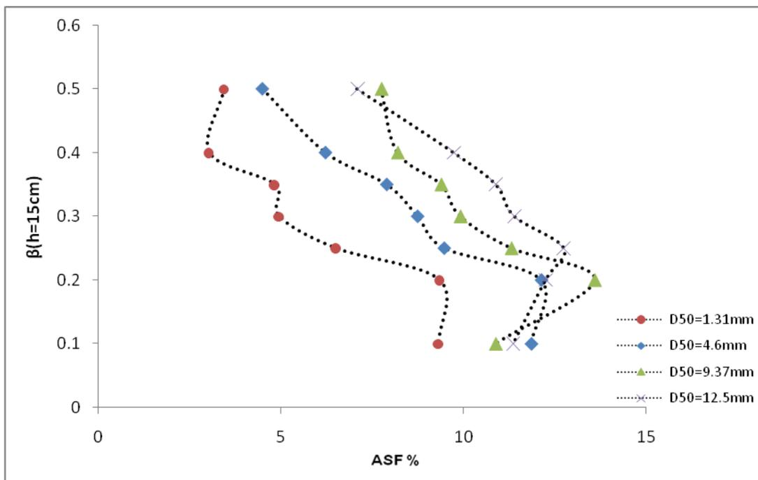
Figure 5: Distribution of shear force (momentum transfer) vs the relative depth  $h = 15\text{cm}$
