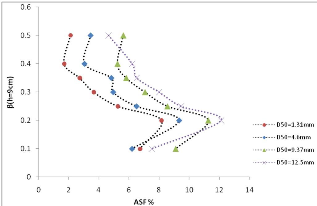
Figure 3: Distribution of shear force (momentum transfer) vs the relative depth h = 9cm
