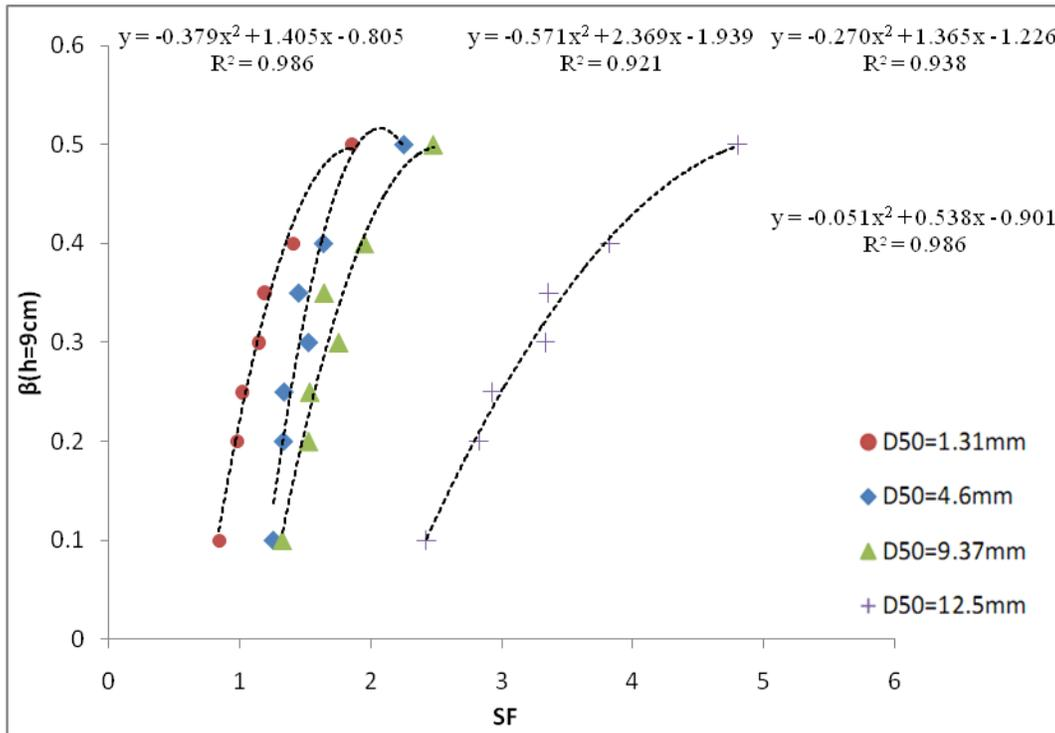
Figure 7: longitudinal shear force at different roughness in ( $h = 9\text{cm}$ )
