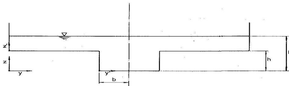
Figure 1: Schematic cross section of the compound channel
