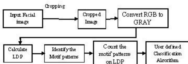
**Figure 1:** Block diagram of age group classification system.
