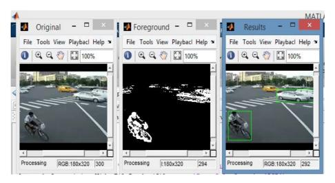
Fig.2 Snapshot of GMM first screen for original video, second for foreground detection, third for tracking.
