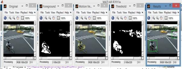
Fig.3 Snapshot of Proposed Method first screen for original video, second for foreground, third for motion vector, fourth for threshold, fifth for tracking.
