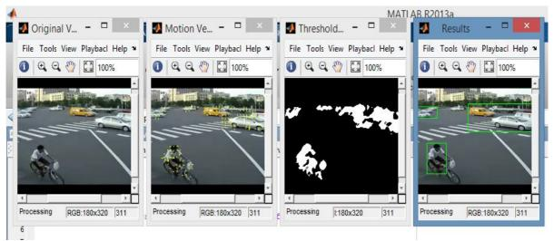
Fig.2 Snapshot of Optical Flow first screen for original video, second for Motion Vector, third for Threshold, fourth for tracking.
