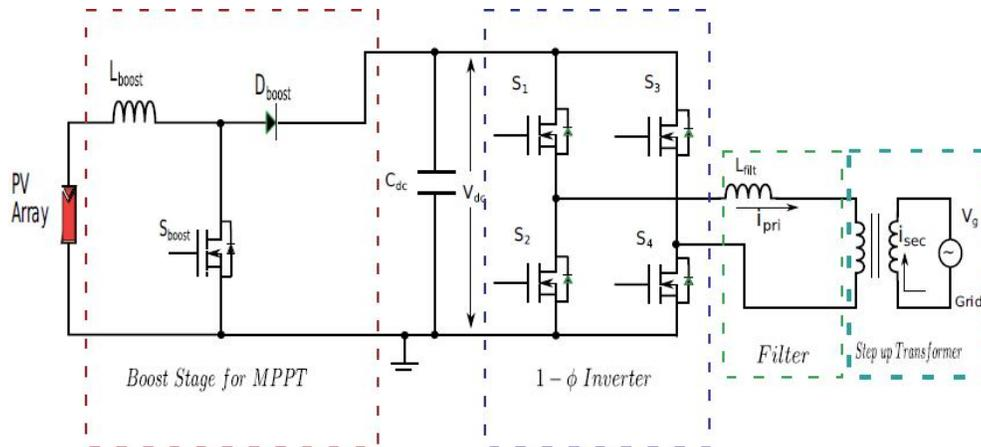
Figure.1 Power circuit topology of 1 $\phi$  PV system.
