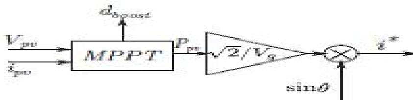
Figure 2. Maximum Power Point Tracking
