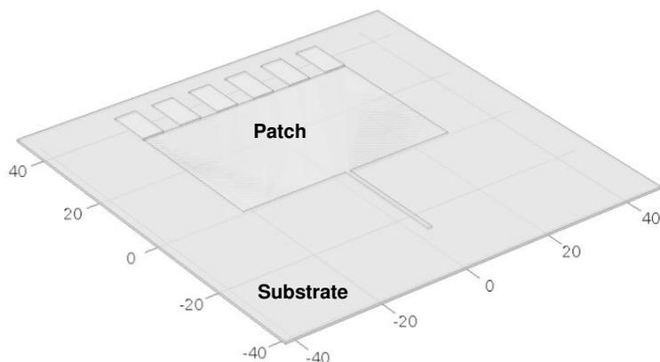
Fig. 2. Geometry of designed microstrip patch antenna.
