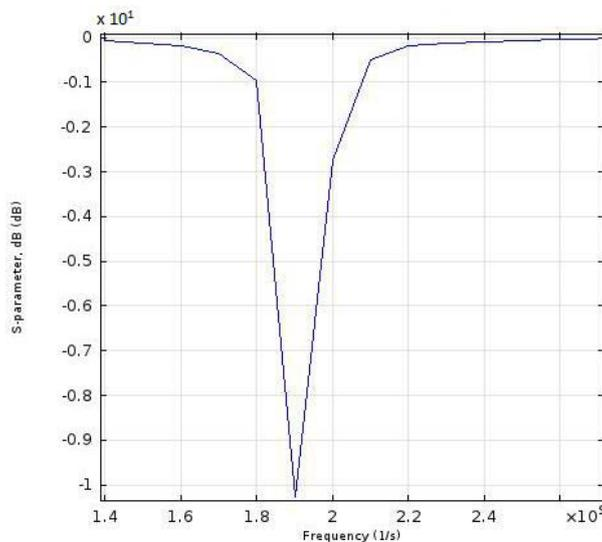
Fig. 4 Return loss vs frequency graph.
