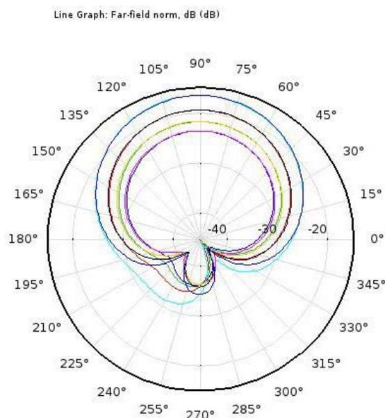
Fig. 6. Line view of the far field radiation of the simulated antenna.
