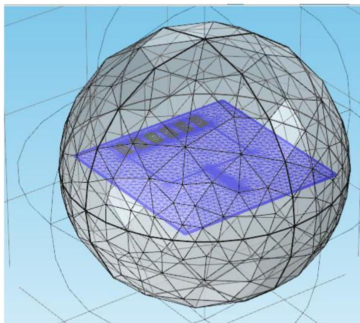
Fig. 2. Mesh formation for the designed microstrip patch antenna.
