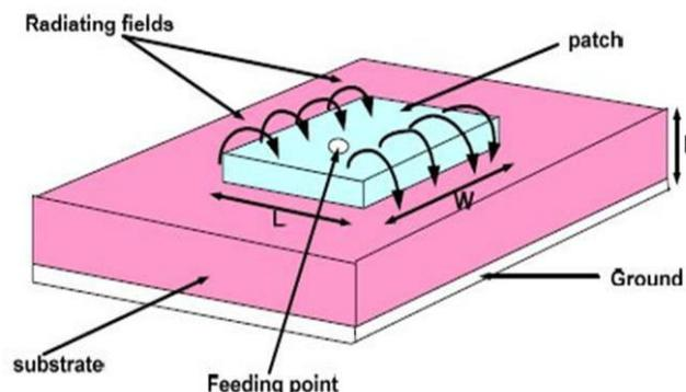
Fig. 1 Schematic of rectangular microstrip patch antenna.
