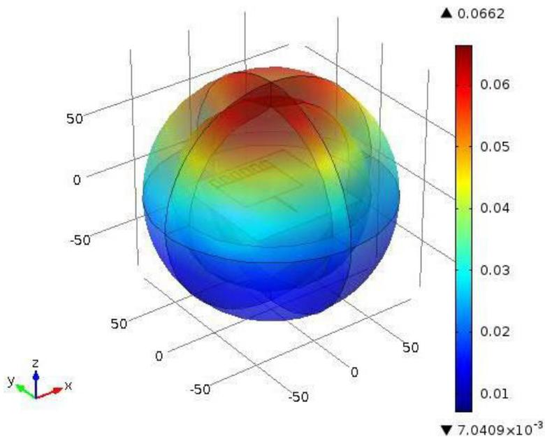
Fig. 5. 3D view of the far field radiation of the simulated antenna.
