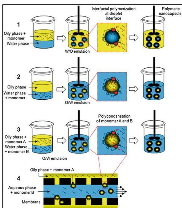
**Figure 8:** Different strategies of Interfacial Polymerization. (1) Monomer introduction onto oily phase (2) Monomer in aqueous phase (3) Monomers introduction in the oily and aqueous phase (4) Polymerization using a membrane reactor device.
