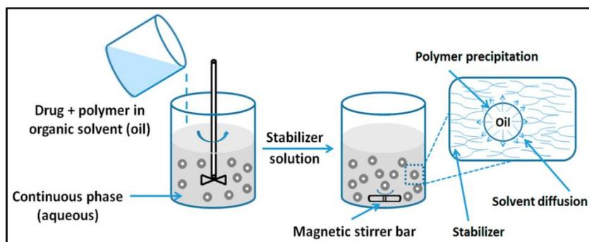
Figure 2: Nanoprecipitation technique.
