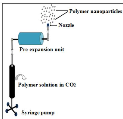
**Figure 6:** Experimental set up for Nanoparticles preparation of Supercritical fluid solution.
