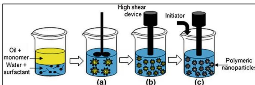
**Figure 7:** Miniemulsion Polymerization Method. (a) Pre-emulsification (b) Nanoemulsification using a high shear device (c) Formation of polymeric nanoparticles upon addition of initiator.
