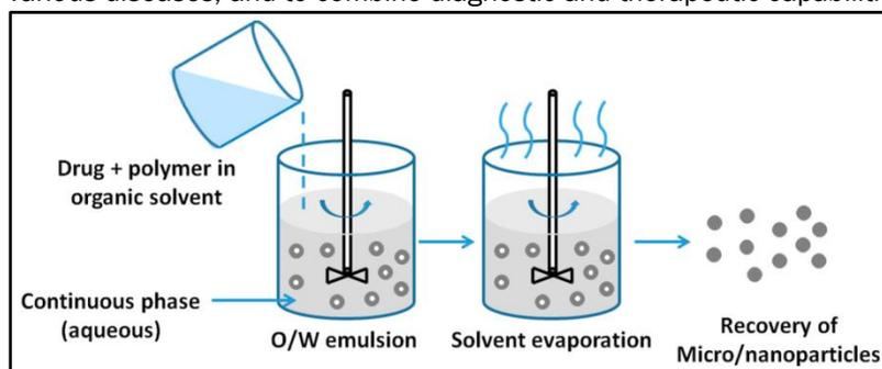
**Figure 1:** Solvent evaporation technique.
