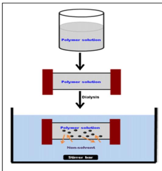
**Figure 5:** Dialysis or osmosis based method for nanoparticles preparation.
