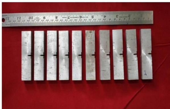
**Figure 2c.** Hardness specimens to perform the hardness test.
