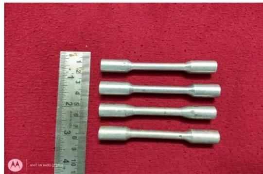
**Figure 2b.** Fracture toughness specimens to perform mechanical failure.
