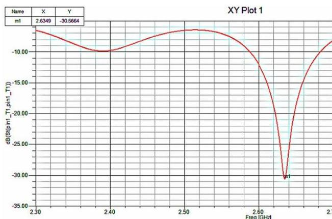
Fig. 9 : Simulation result of S11 for antenna at 2.63GHz
