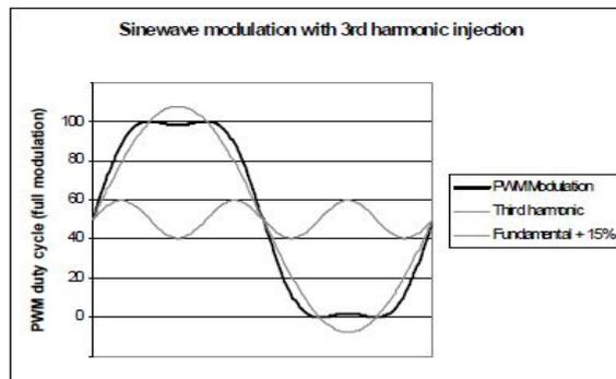
Fig. 4. Effect of third harmonic injection in reference sine wave
