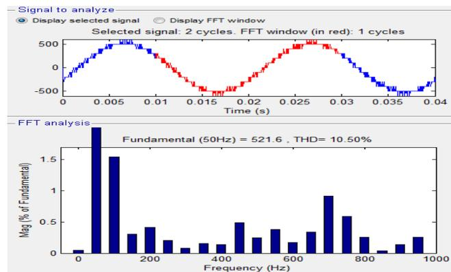
Fig. 11. THD Analysis of line to line voltage without third harmonics injection
