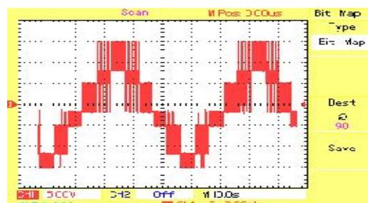
Fig. 13: Seven Level Output Obtained
