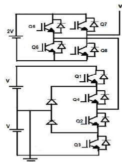
Fig. 1. Circuit Diagram of Hybrid NPC-HB Topology for Single Phase
