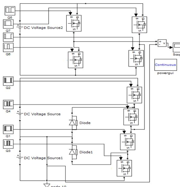
Fig. 5. Simulation Diagram to Test the Operation of 7 Level Inverter in MATLAB/SIMULINK
