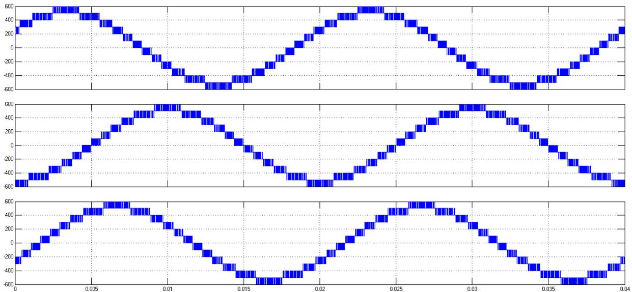
Fig. 9. 13 level line to line voltage with third harmonic injection
