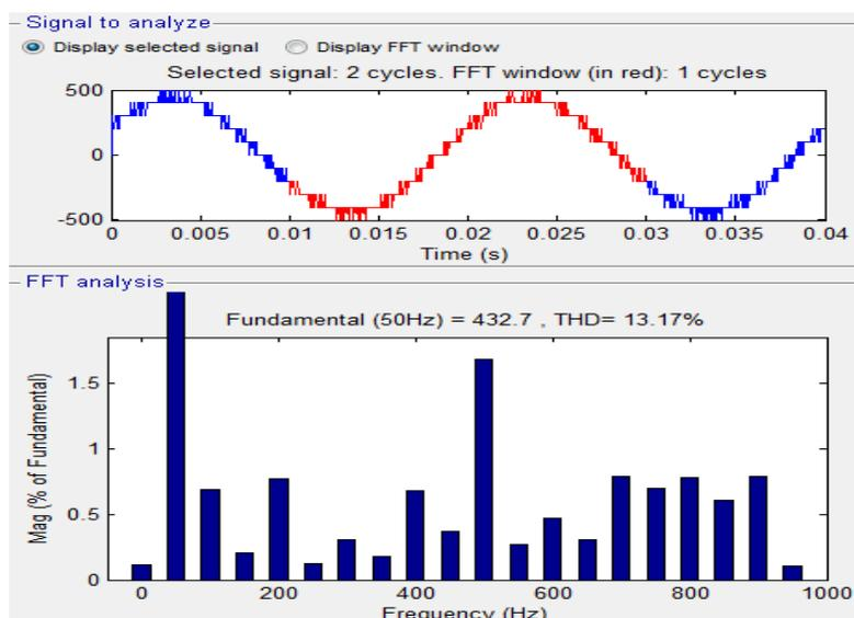
Fig. 10. THD Analysis of line to line voltage without third harmonics injection
