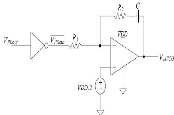
Fig 3 Active PI loop filter
