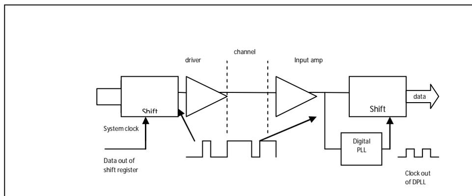
Fig. 1 block diagram of a communication system using a DPLL for the generation of a clock signal
