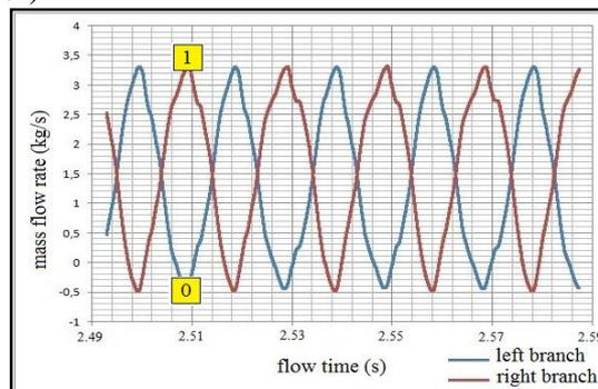
Fig.2. The mass flow as a function of time (s) To branches (right and left).
