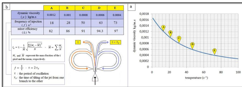
Fig.7. (a) The curve of the viscosity variation dynamics of water as a function of temperature; (b) The efficiency of the micro-mixer for different injection frequencies.
