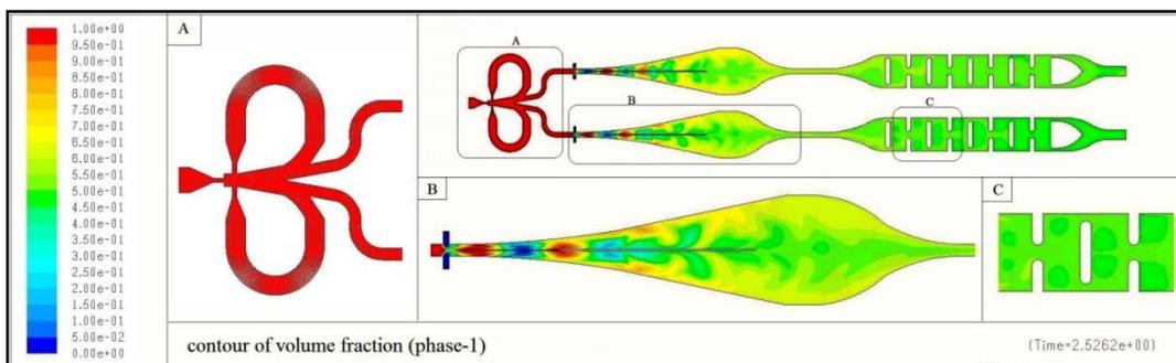
Fig.6.Represents the contour of the mass fraction in the micro-mixer.
