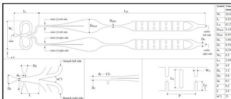
Fig.1. Description of the simulated fluid mixer geometry.
