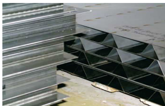
Figure 2: Stock of Doltrac floor assemblies with sandwich structure which profiles are of continuous ‘V’
