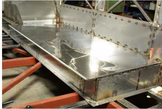
Figure 3: An experimental, sandwich-panel bus floor element, in grade 1.4003, assembled using laser welding
