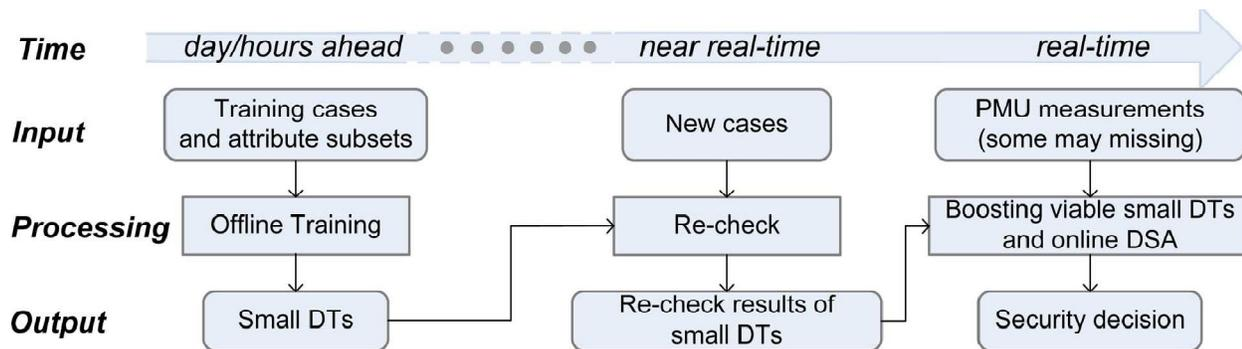
Three-stage ensemble DT-based approach to online DSA with missing PMU measurements.:
