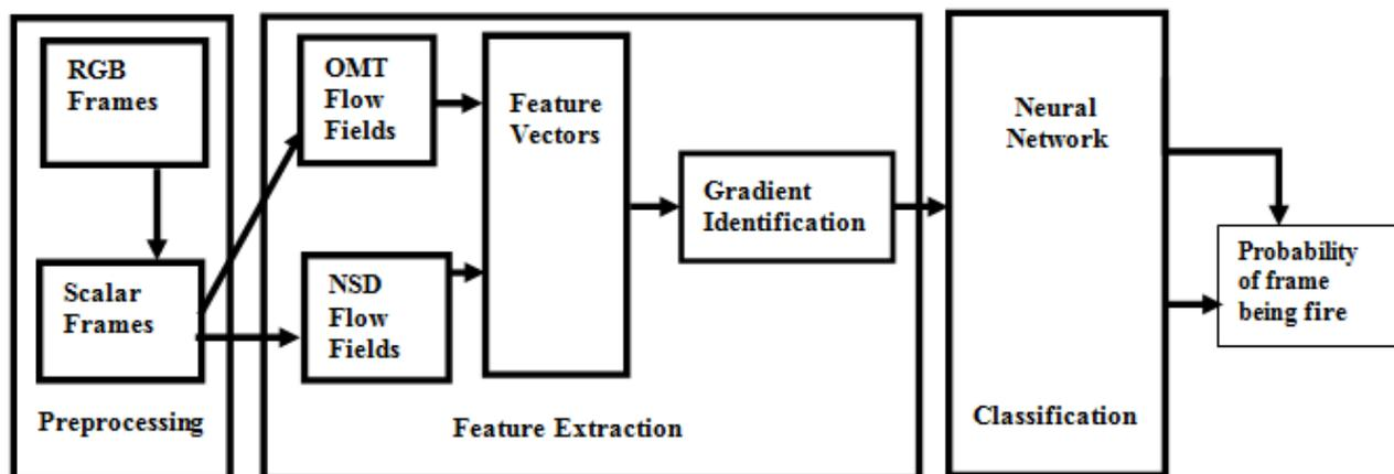
Fig. 1. Flame Detection System
