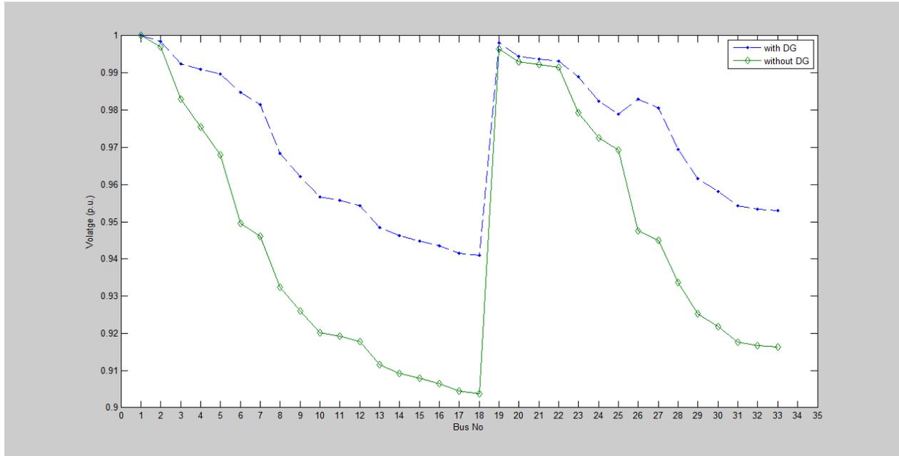
Fig 2. Variation of voltage profile for 33-bus Radial Distribution System
