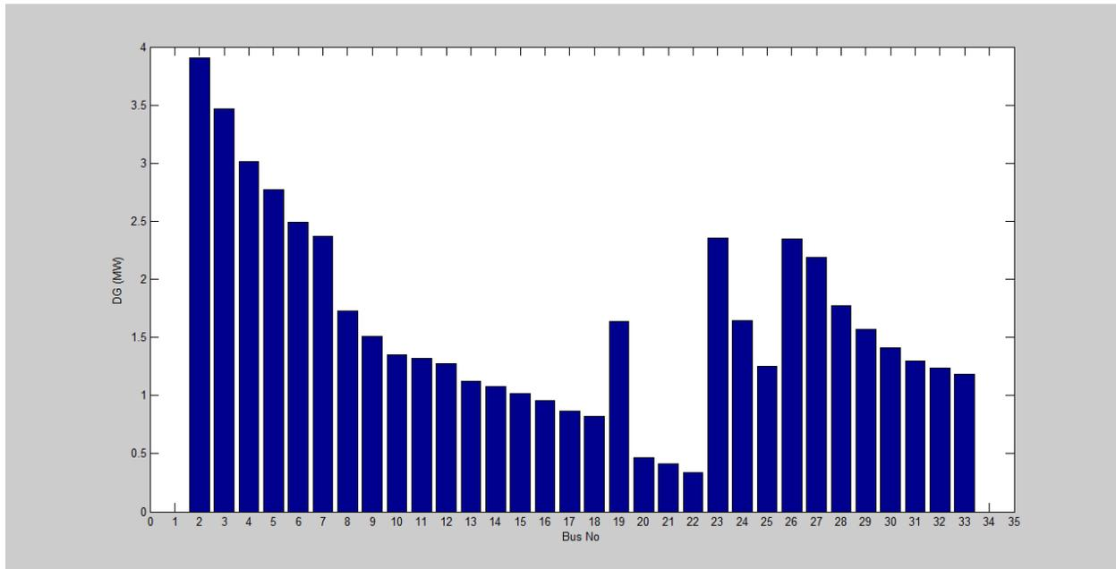
**Fig1. Optimum size of DG at each of 33-bus Radial Distribution System**
